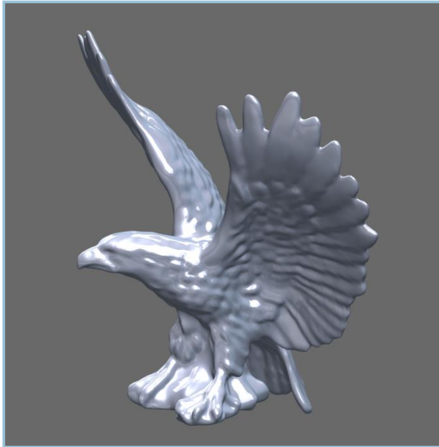
The eagle reference mesh retopologized and then converted to CAD
